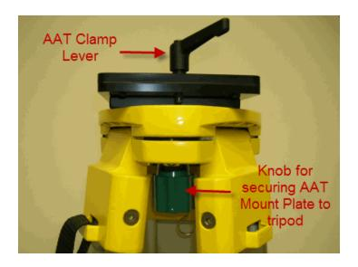
c. Slide AAT into mount on tripod and clamp into position using lever
