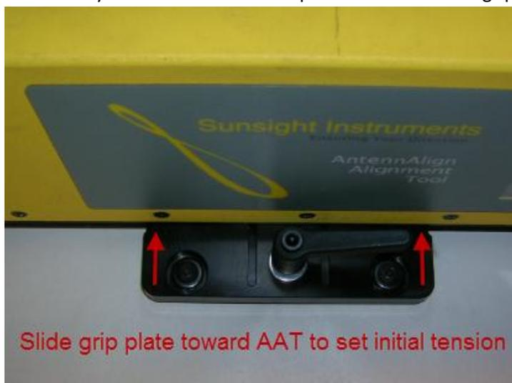
4. Slide AAT side-to-side in the grip sub-assembly to determine the grip clamp tension. No play should be detected between the AAT and the grip clamp and little to no friction should be felt when the AAT is sliding in the mount.
